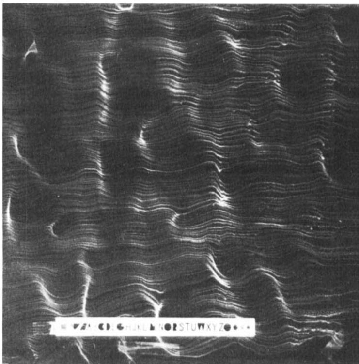
FIGURE 24. The spanwise coherence of the large eddies in the wake of a circular cylinder at  $\bar{x} \approx 600$  and  $Re_\theta = 600$ .
