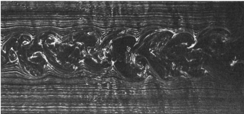
FIGURE 23. Large coherent structures photographed in the wake of the flat plate with no forcing.  $\bar{x} \approx 500$  and  $Re_\theta = 600$ .
